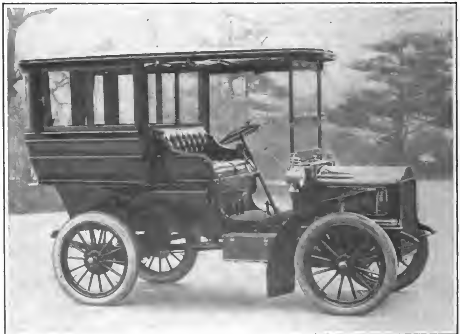
The engraving above is from a photograph of a 1905 model White steam car, fitted with limousine body, to the order of Charles A. Starbuck, of New York, to whom it was delivered last week. The interior seats four persons comfortably, is handsomely upholstered in Russian leather, and is illuminated at night by means of electricity supplied from a storage battery on the car. The windows are fitted with black silk spring roller curtains.
